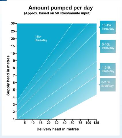
Distance pumped is dependent on delivery head and pipe friction - consult pipe manufacturer's friction chart. If more water is required, multiple pump installations can be adopted.
